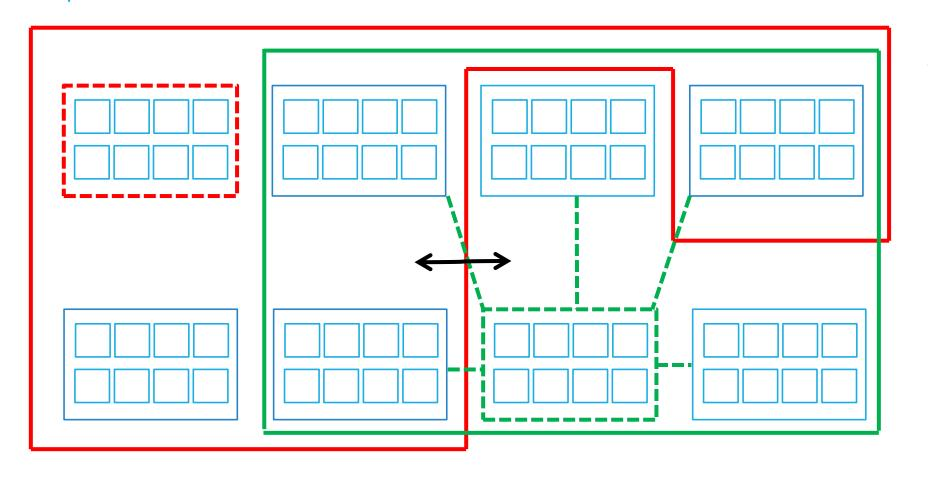
At the 4<sup>th</sup> level, the first group of directly connected CPUs balances load with the other groups of directly connected CPUs
