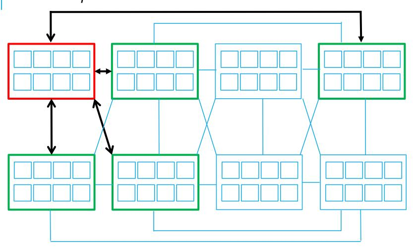
At the 3<sup>rd</sup> level, the first CPU balances load with directly connected CPUS
